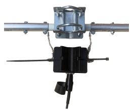
Your co-axial cable can now be fitted to the matching transformer with a PL259 connector. Seal the connector against moisture using the self amalgamating tape. Remove the backing layer and wrap the tape tightly from the socket to the plug.
