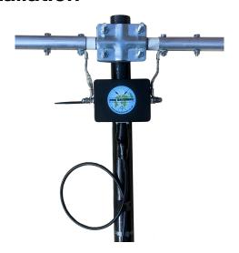
Form a small loop prior to taping the coax cable to the support mast using PVC insulating tape. If you are using a rotator, ensure there is enough slack in the cable to allow the mast to rotate without restriction.
