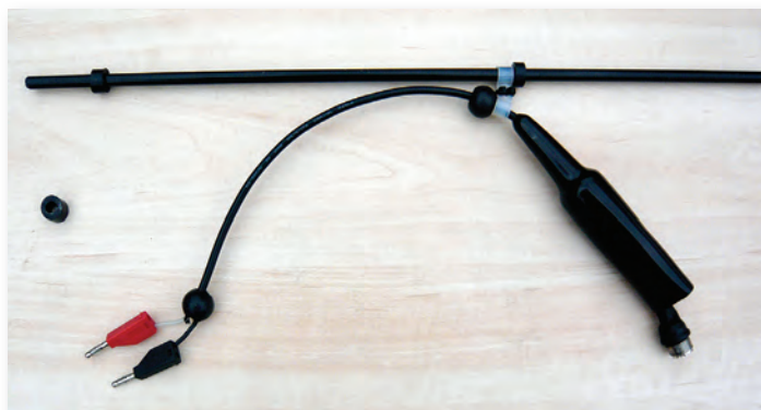
Fig. 6: A small modification to the leads was needed to reduce the tendency for the 'earthy' side plug to pull out.
